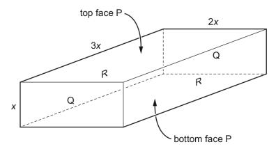
Electrical contact can be made to the block between opposite pairs of faces (for example, between the faces labelled R).
