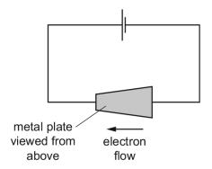
Electrons move clockwise around the circuit.
