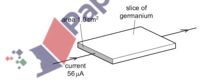
What is the average drift velocity of the charge carriers in the germanium?
